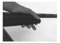
Screw tha magazine cap and hand tighten.
