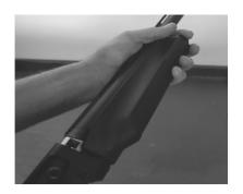
1-Unscrew the magazine cap and take out the forend and barrel group by sliding forward.
