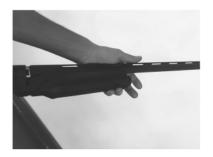
Install the fore end on the barrel-breech unit and Fit the breech extension onto the receiver by sliding the fore-end along the magazine tube.
