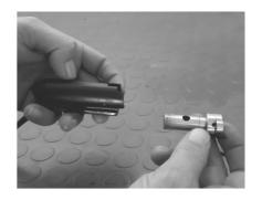
4-Remove the locking head pin from the bolt and remove the bolt locking head from the bolt.
