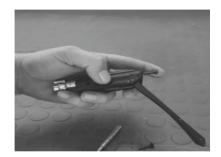
3-Remove the firing pin retaining pin from the bolt assembly, while holding the firing pin and firing pin spring in place
