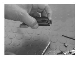
5-Remove the inertia spring from its seat in the bolt.
