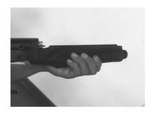
Unscrew the fore-end cap and remove from the magazine tube
