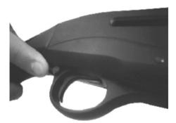
3. When you are ready to fire the gun, press the safety button to the "off" position so that the safety protrudes from the left side of the gun and the RED BAND MARKING IS SHOWING.
