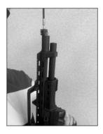
8- With the fore-end in the back position, clean the inside of the barrel with suitable cleaning kits.
