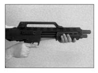
5- Push the forend forward and close the action so that the first shell enters the chamber. Get the safety OFF and your gun is now ready to fire.
