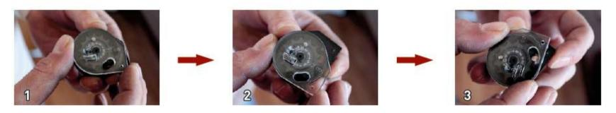
Rotate the front cover in the direction of the arrow (clockwise)
