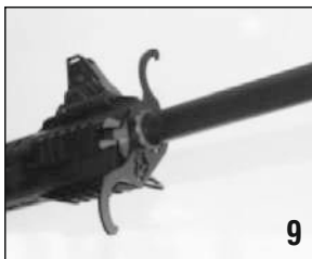
9. Loosen the Fore-End Nut (20) using the proper key.
