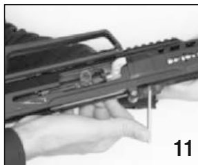
11. Loosen these 2 screws with 4 mm allen key.
