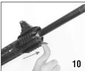
10. Loosen the items 19 and 20 with pulling the swivel stud.
