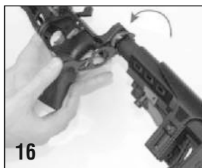
16. Loosen the stock support nut (3) towards to the arrow with the key.
