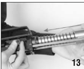
13. Remove the action bar (100) as shown at the picture.
