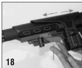
18. With this red part, you can adjust the stock and also adjust the cheek distance with loosen the screw on the right.
