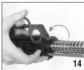
14. Remove the retaining pin (84) towards the arrow.
