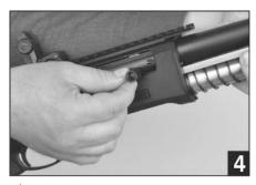
**4)** Remove bolt handle by pushing bolt carrier. (**Figure 4**)
