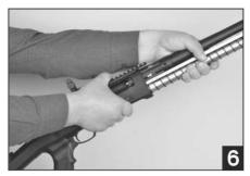
**6)** Remove the barrel by pushing forward. (**Figure 6**)
