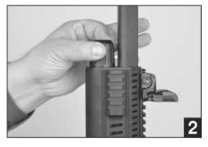
2) Remove the magazine cap counter clockwise (**Figure 2**)
