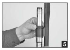
**5)** Remove the barrel nut counter clockwise. (**Figure 5**)
